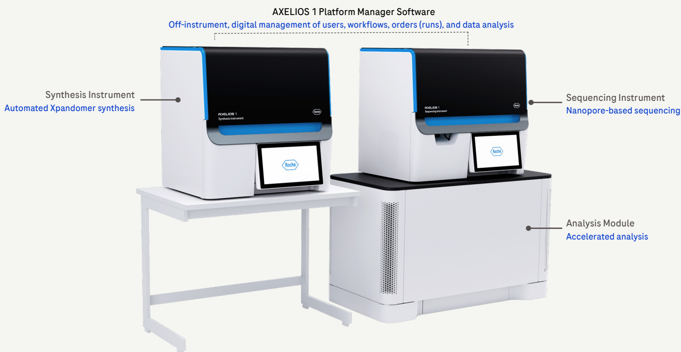
Figure 1. The AXELIOS 1 Platform for next-generation sequencing. The synthesis instrument offers the flexibility to synthesize one to four Xpandomer pools in parallel in up to 4 h, independently from sequencing. The sequencing instrument employs a reusable CMOS-based sensor module and standardized reagents, thereby enabling uninterrupted sequencing of up to four Xpandomer pools in 16 h of sequencing time (not including pre-sequencing setup and post-run clean up). The analysis module provides high-accuracy, near real-time primary / post-primary data analysis (base calling, as well as demultiplexing, intramolecular consensus, and reference-based alignment for SBX-D). The AXELIOS 1 Platform Manager Software provides an intuitive user interface for integrated, off-instrument management of users, synthesis and sequencing orders (runs), and data analysis. The platform supports a wide range of methods through flexible read lengths and tunable throughput (sequencing times and / or batch sizes).
