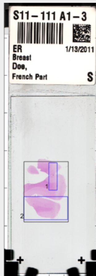
Figure 5. Multiple AOIs (blue rectangles) are merged into a single rectangular BIF-image (black outline). The BIF-image approximates the convex hull of all AOIs. Areas of the BIF-image not scanned as part of any of the AOIs are represented in the BIF-file using empty JPEG-tiles (zero length). The upper left corner of each AOI is encoded in the Attributes of the AoiOrigin child nodes <AOI1> through <AOIN>. AoiOrigin always falls online boundaries.
