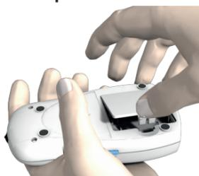
Open the battery compartment on the back of the meter.
