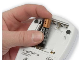
Insert 4 AAA alkaline batteries according to the diagram inside the battery compartment.
