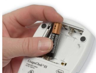
Insert 4 AAA alkaline batteries according to the diagram inside the battery compartment.
