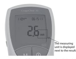
To reset the measuring unit to INR, follow the instructions in the *Advanced Features* section of the *CoaguChek XS System User Manual*, version 9.0 and higher, or call the Roche Diagnostics Technical Service Center at 1-800-428-4674 for assistance, if the result is displayed in %Q or Sec.
