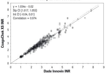
Accuracy: 700 capillary samples were collected from 357 outpatients at three external sites. Capillary blood samples were assayed on the CoaguChek XS meter with the CoaguChek XS PT Test and venous plasma samples were measured on a Dade Sysmex 560 Analyzer using Dade Innovin (ISI = 1.02) The results comparison is as follows:
