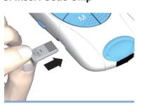
Make sure the meter is off. With the code number facing up, insert the code chip into
