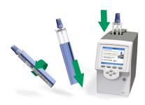
7 Once the negative control result is accepted, choose **Confirm**. Then remove and discard the assay tube.
