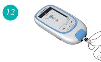
The test strip symbol prompts you to insert a test strip.
