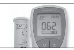
5. An hourglass appears as the meter warms up, which takes up to 30 seconds.6. When the meter is warmed up, a flashing test strip and blood drop symbol appear and the meter begins a countdown. You have 180 seconds to apply blood
